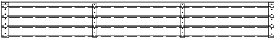
RP01 | ROOF PANEL - W2A02182 (x1) | 1/16"x1/16"x1/16" (40x287x2165)
