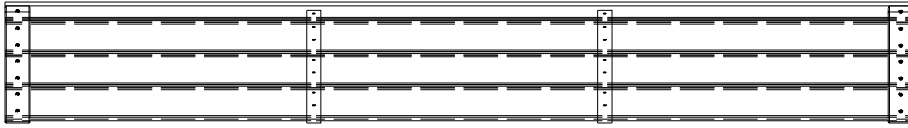
RP01 | ROOF PANEL - W2A02182 (x1) | 1/16"x1/16"x1/16" (40x287x2165)
